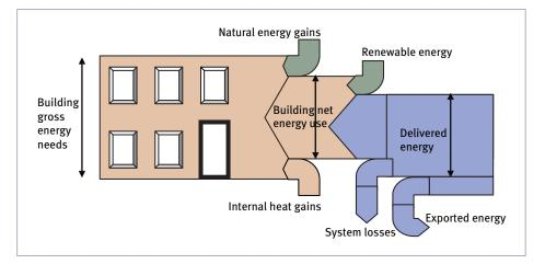
Figure III. How energy flows are linked in buildings<sup>a</sup>
